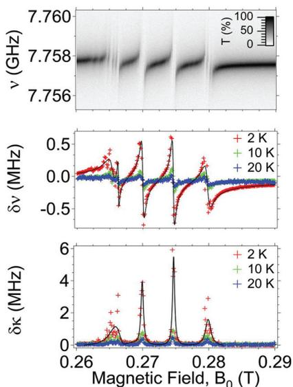
**Fig. 5** (Upper panel) Transmission spectral map measured at 2 K for a diluted (2%) and deuterated single crystal of  $\text{Cu}(\text{mnt})_2$  ( $P_{\text{in}} = -63$  dBm,  $\theta = 0^\circ$ ). (Middle panel) Field dependence of the shift of the resonator frequency and (lower panel) the relative variation of the linewidth. Data taken at 2, 10 and 20 K are shown for comparison. Solid lines display the fitting curve calculated from eqn (1a) and (1b).
