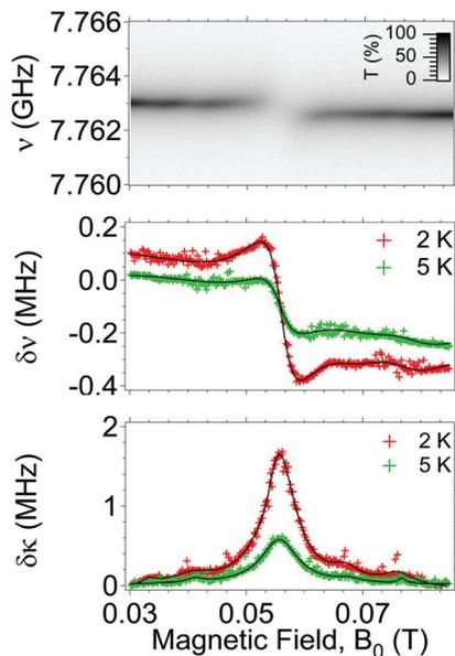
**Fig. 7** (Upper panel) Transmission spectral map measured at 2 K for a diluted (3%) single crystal of Dy(trensall) ( $P_{\text{in}} = -43$  dBm,  $\theta = 90^\circ$ ). (Middle panel) Field dependence of the shift of the resonator frequency and (lower panel) variation of the linewidth. Data taken at 2 and 5 K are shown for comparison. Solid lines display the fitted curve calculated from eqn (1a) and (1b).
