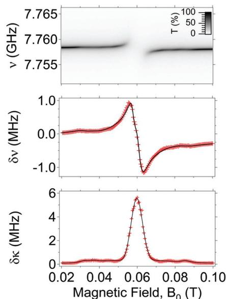
**Fig. 6** (Upper panel) Transmission spectral map measured at 2 K for a diluted (10%)  $[\text{ErPc}_2]^- \text{TBA}^+$  single crystal ( $P_{\text{in}} = -43$  dBm,  $\theta = 90^\circ$ ). (Middle panel) Field dependence of the shift of the resonator frequency and (lower panel) variation of the linewidth. Solid lines display the fitting curve calculated from eqn (1a) and (1b).
