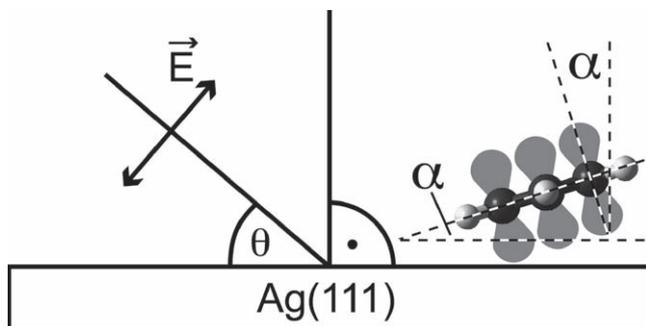
**Scheme 3.** The geometry of the NEXAFS setup. The incidence angle  $\theta$  defines the direction of the X-ray beam with respect to the sample surface. The adsorption angle  $\alpha$  describes the orientation of a molecular moiety with respect to the underlying surface. In the displayed example of a benzene ring (carbon atoms in black, hydrogen atoms in white),  $\alpha$  is the angle between the direction of the  $\pi$ -system (gray lobes) and the surface normal.
