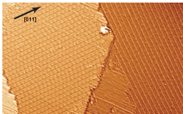
Figure 2. STM overview ( 650 \text{ \AA} \times 400 \text{ \AA} ) displaying extended and highly ordered domains of thermally stable P1/C1 mixed phase. Two rotational domains ( 90^\circ separation based on substrate symmetry) are here separated by a single atomic step in the Cu(100) substrate.
