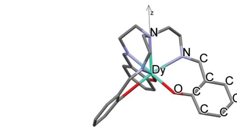
Fig. 4 X-ray structure of the  $\text{Dy}(\text{trensall})$  molecule. Colour scheme: Dy, cyan; O, red; N, violet; C, grey. H atoms are omitted for clarity.
