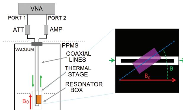
**Fig. 1** (Left) Schematic diagram of the experimental set-up. (Right) Top view of the YBCO coplanar resonator (black) with a crystal loaded on top (purple). The red arrow indicates the applied magnetic field, while the green ones indicate the propagation of the TEM microwave signal.  $\theta$  is the angle between the static magnetic field and the crystal *c*-axis.
