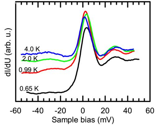
FIG. 8. (Color online) Differential conductance  $dI/dU$  of Ni<sub>2</sub>- $\beta$  measured at different temperatures. Sidebands at 30 mV are surrounding the Kondo resonance at zero bias. Feedback conditions:  $U = 50 \text{ mV}$ ,  $I = 1 \text{ nA}$ , 2 mV modulation.
