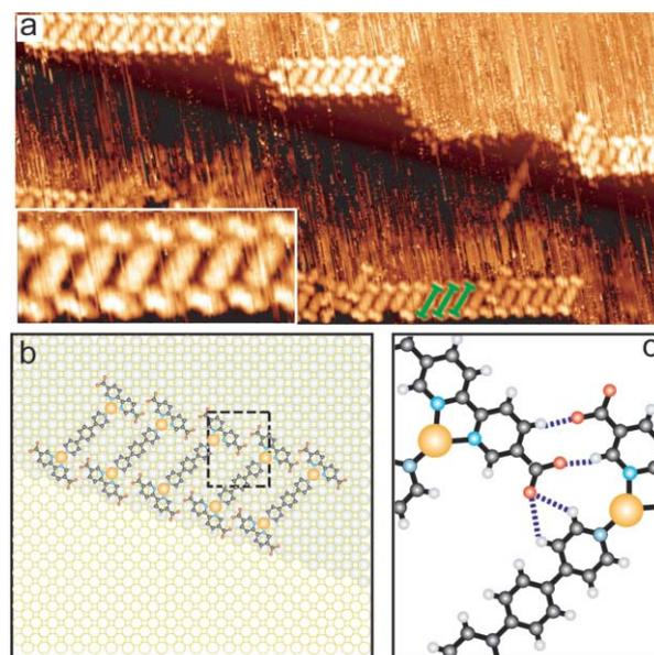
**Fig. 2** (a) STM topograph ( $44 \times 22$  nm) showing the supramolecular organization of the dumbbells at step edges, green dumbbells illustrate the ladder structure. (b) Molecular structural model of the ladder phase with respect to the substrate lattice, color change of the substrate showing the step. (c) Enlarged view of the rectangular area of (b), the possible hydrogen bonds shown by dotted lines. Color code same as Fig. 1.
