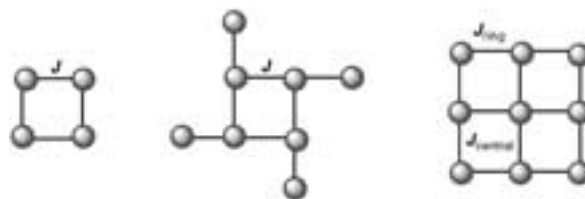
Figure 22. Definition of the coupling constants J in [2 \times 2] arrays (left), [2 \times 2] "pin-wheel" arrays (middle), and [3 \times 3] arrays (right).
